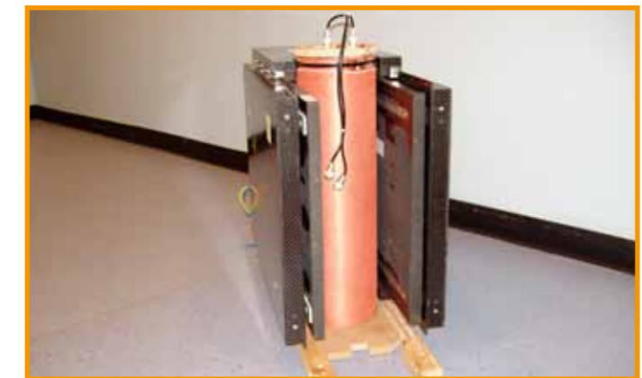
Final magnet ready for lab test
