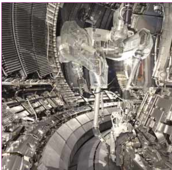
A remote handling arm inside the JET torus.
