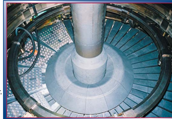
Part of the new MAST graphite divertor.
