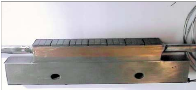
The baffle mock-up, shown here, endured 1000 cycles at 5MW/m 2 and 90 cycles at 7MW/m 2 during heat flux testing
