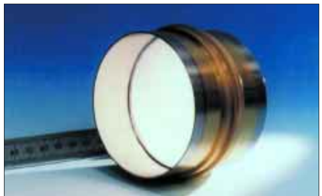
An STG bonded CVD diamond window mounted into a gyrotron wave-guide assembly—a window capable of being baked at 450°C and withstand 144 GHz, CW radiation at a power of 1 MW.
