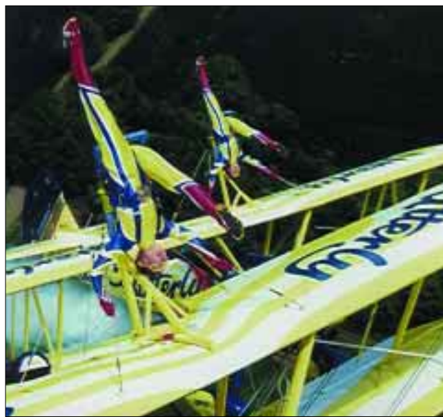
'Wing walking' pylon designed by Acro Aeronautical for the 2001 'Utterly Butterfly' aerobatic team. The wing rider can rotate about the forward and vertical axes. The aircraft is a Boeing Stearman.
