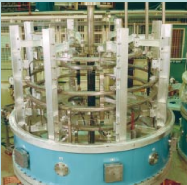
PF Coils in the START machine at Culham
