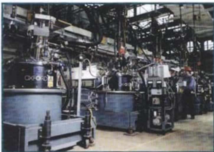
Oxford Instruments' gyrotron magnets at the UKAEA Culham Science Centre
