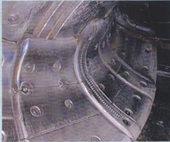
A segment of the COMPASS-D graphite 'divertor tiles', fitted with an array of probes to measure heat flux and local plasma properties.
